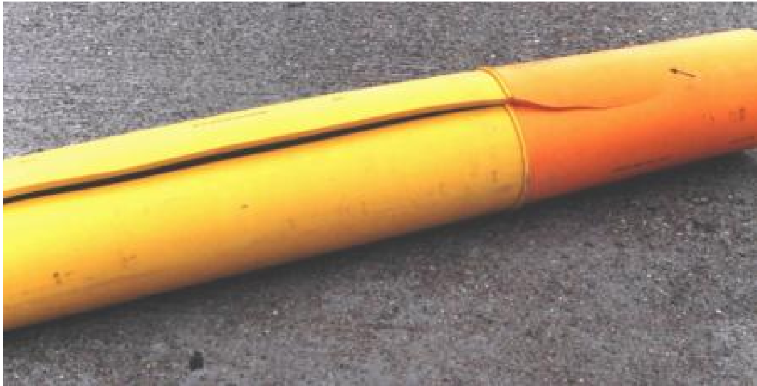
RCP arrest in PE100 pipe
